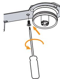
1-6. REMOVE THE MODULE FROM C-LOCK
